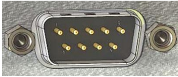
Figure 3-13. Laser Marking Module XY2-100: 9-Pin Male Pinouts
