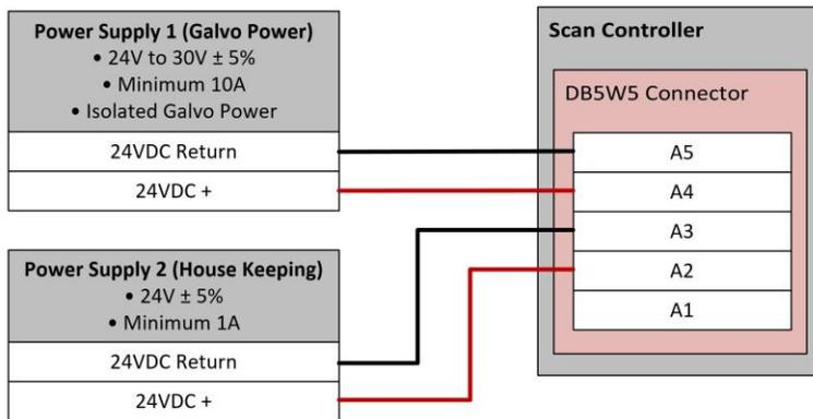
Figure 6-5 Power Supply Configuration - YLS Laser (with Hardwire Interface)
