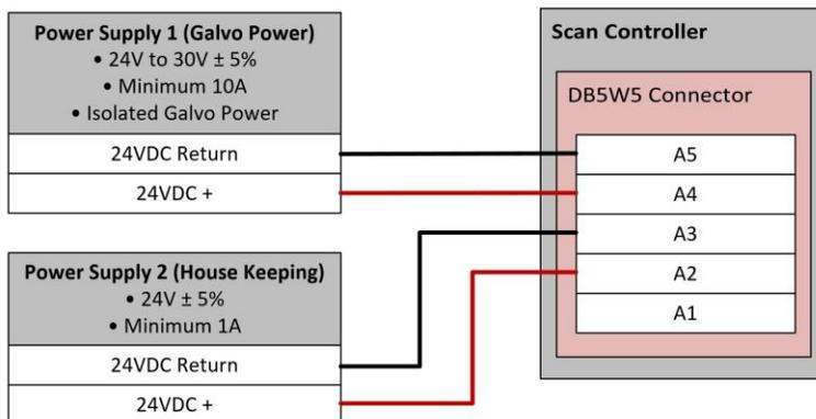
Figure 6-17 Scanner with YLP Power Supply Configuration
