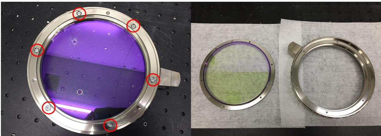
5. Insert the replacement protective window glass into the frame. Be sure that the sealing O-rings are properly seated prior to placing the protective window glass. See Figure 9-6.
