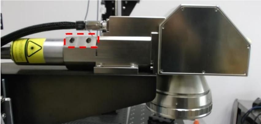
3. Remove the cap that covers the collimator, carefully insert the collimator into the collimator holder on the scanner, and gently push it all the way.
