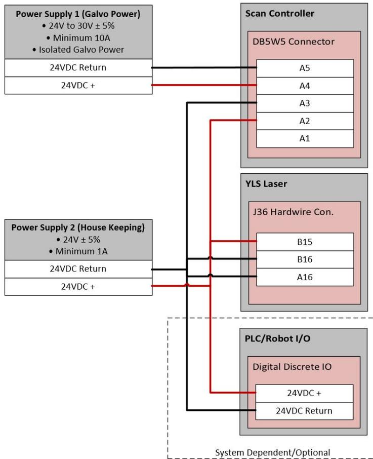
Figure 6-16 Scanner with YLR Power Supply Configuration
