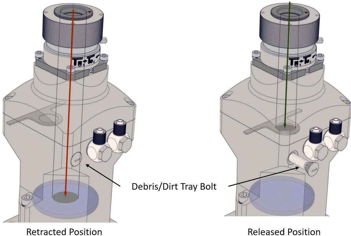
To release or retract the debris tray, simply turn the debris tray bolt accordingly.
