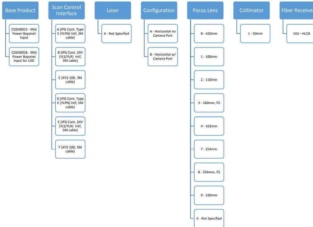
Figure 2-5 Mid-Power Scanner with Collimator Input Part Number Configurations
