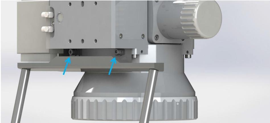
2. Adjust the angle of the air knife by loosening clamps (see purple arrows in Figure 5-5).
