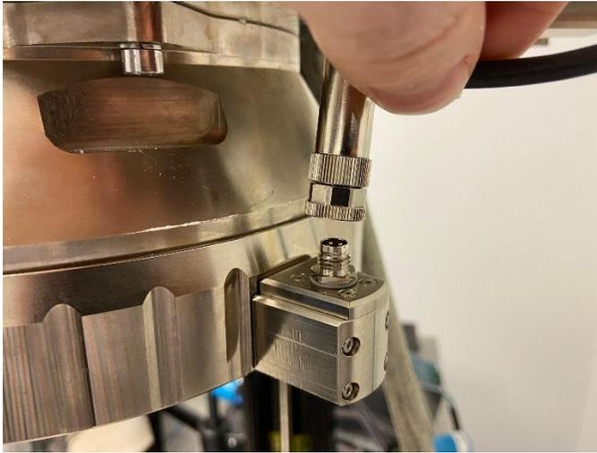
2. Rotate the Window Assembly on the scan head clockwise (if looking at the front of the scanner) to remove it from the focus lens assembly.
