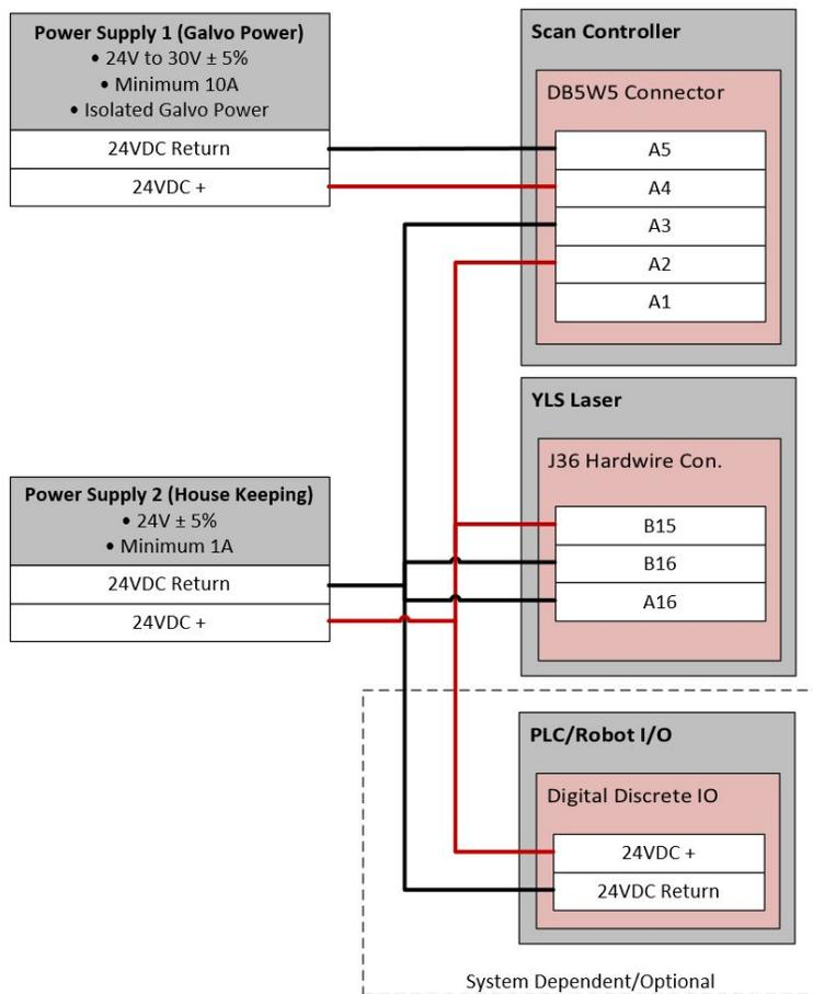
Figure 6-6 Power Supply Configuration - YLS Laser (with Fieldbus Interface)
