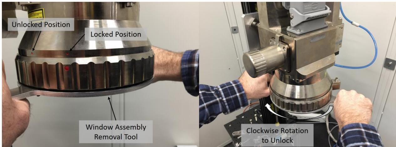
3. With the Window Assembly unlocked and rotated clockwise, the Window Assembly will drop off the lens assembly (see Figure 9-4).
