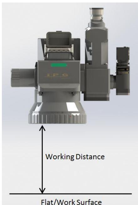
9. Using IPGScan software, mark a cross (as seen in Figure 5-9) at 0, 0, 0 in the scanners Field of View (FOV). Once marked, make sure the head is not moved from this position until camera setup is complete.
