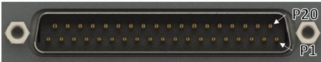
I/O signals out of this connector are either 3.3VTTL or RS422 compatible. Bidirectional I/O signals are not isolated and IPG does not recommend direct connection with them. To properly integrate the Scan Controller into an automated system, an External Interface Device such as the 24V Interface, Extended IO Interface, or Motion Interface should be utilized. Please refer to the External Interface Board User Guide (DOCOXUGSCNXX0002) for additional details.
